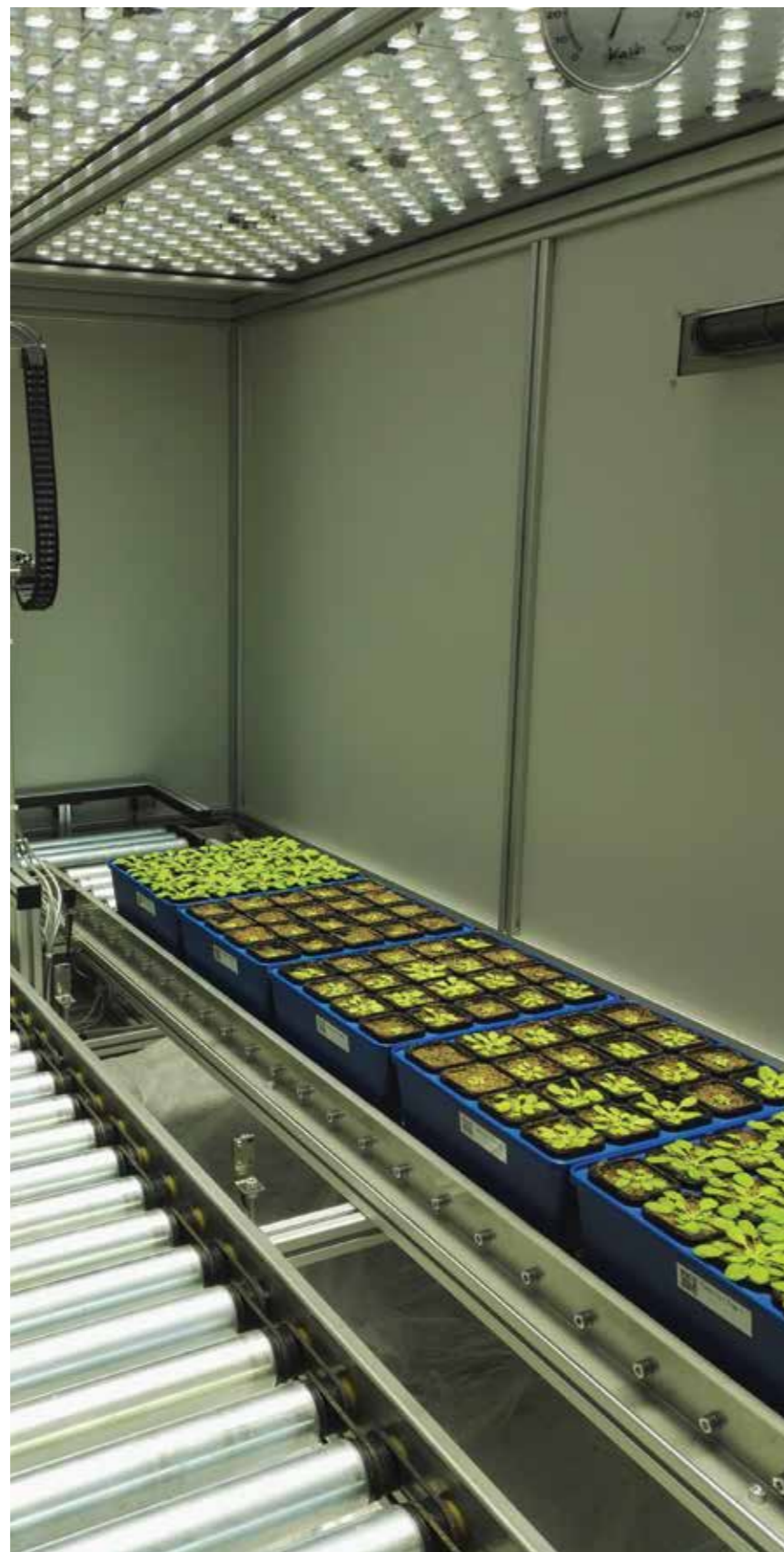
A phytoscope is an imaging device that analyses plant growth and physiology. The plants are measured and images are taken of them automatically, after which the computer calculates the height, width and, for example, the surface area and shape of the rosette based on the images.
